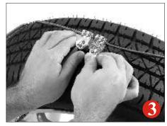
Reach around each side of the tire and grasp both ends of the non-split side cable (that is furthest away from you). Pull both ends to the top of the tire so the fasteners can be seen and manipulated more easily. Connect the inside fastener.
