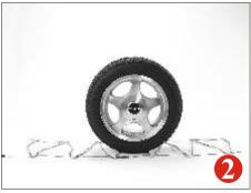
Move the chain in a sweeping motion under the vehicle so the open mid-section is positioned up against the backside of the tire. This sweeping motion can best be done while kneeling in front of the tire.
