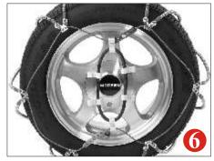
Attach tensioner to take up additional slack. To make this simpler, attach the first hook at the "12 o´clock" position, the next hook opposite at the "6 o´clock" position and so forth.
