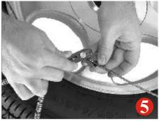
Connect the bottom fastener. In order to close the outside fasteners, they must be at an angle to each other.
