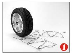
Park vehicle on firm, level ground and away from the flow of traffic. Set the emergency brake. Remove any wheel covers. Chains should be installed on drive wheels. Lay the cable chain on the ground with smooth side (TIRE SIDE) of the crossmember hooks up.
