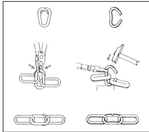
**GB** Repair the broken chains with the repair links kit to avoid all possible damages to the car's body.
