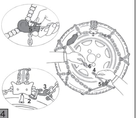
**GB** Thread the tension cable (4) through the stop device (5). Hook the plastic hook (6) with the ring of the tensioning cable (4). The chain automatically tensions and centres, so there is no need to stop after you leave.
